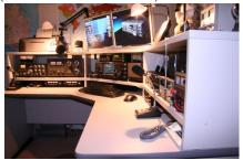
the top of the heap is the **base station**. These rigs sit on a desk or bench, have their own power supplies, can put out 1000+ watts using a separate amplifier, have very sophisticated reception and transmission controls, and really-really pretty lights and dials and knobs and switches and stuff.
